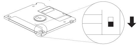
• To allow writing onto a diskette, slide the write-protect tab to cover the protect slot, as shown in the following illustration.
